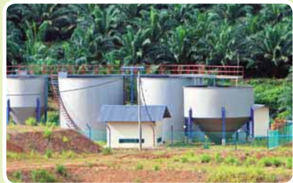
Among the steps taken by the Group to ensure biochemical oxygen demand are at permissible levels, is the implementation of bioflow plants at oil mills
